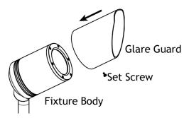
Install the glare guard back onto the fixture body and secure with previously removed set screw. Hand tighten until snug.
