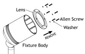
Loosen Allen screws to remove the washers and the lens from the fixture body.
