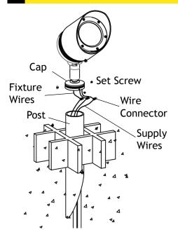
Allow enough wire from the fixture for adjustment purposes. Connect the wires from the fixture into the wiring terminal. The white wire goes to the "Neutral" terminal; the black wire goes to the "Live" terminal; and the green wire goes to the "Ground" terminal. Fix them in place with the connector screws.
