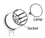
Insert the bulb with the correct wattage and type marked on the fixture label and screw tightly into place.
