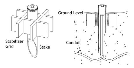
Dig a hole in the ground for the conduit runs and the stake. Install the conduit. Slide the stabilizer grid onto the stake and secure with the screws. Place the stake over the conduit runs. Backfill against the mounting stake.
