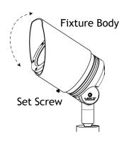
Loosen the screw at the joint and adjust the fixture body to the desired direction. Once the desired direction is achieved, tighten the set screw until snug.
