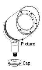
Thread the cap onto the fixture body and hand tighten until snug.
