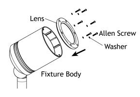
Place the lens back onto the fixture body and secure with the Allen screws and washers. Tighten until snug.
