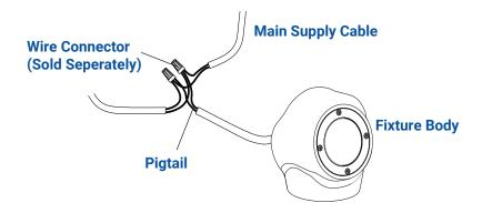
Place fixture body on your desired location. Strip both leads from luminaire pigtail. Using two UL listed wire connectors (sold separately), connect the leads from the fixture body to main supply cable leads. Make this connection at least 10 feet outside of the water.
