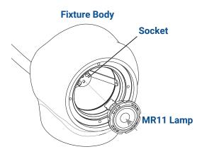
Insert MR11 lamp with correct wattage and type marked on fixture label.
