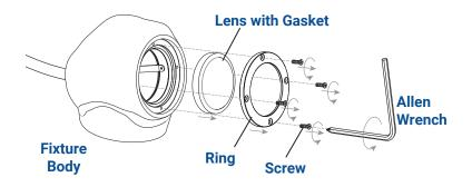
By using the screwdriver end of the Allen wrench, loosen four screws and remove them from the fixture body. Remove the ring and the lens with gasket.
