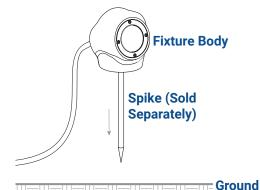
Determine the desired location for mounting the fixture body. Insert the spike into the soil completely.
