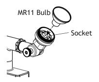
Insert the MR11 bulb with correct wattage and type marked on fixture label and secure into place.
