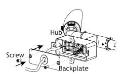
Carefully tuck all the extra wire inside of the hub and place the backplate onto the hub. Secure by using the previously removed screws. Tighten with a screwdriver.
