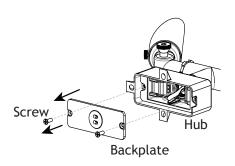
Take off the backplate from the hub by removing the screws on the back.
