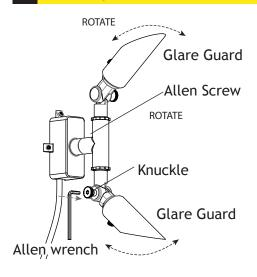
Using an Allen wrench, loosen the knuckle and adjust the fixture up and down to your desired direction.
