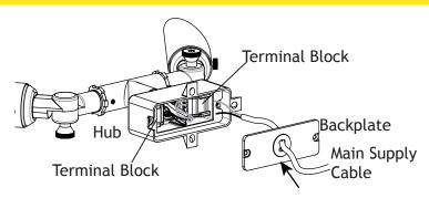
Pass the main supply cable through the center hole on the backplate.
