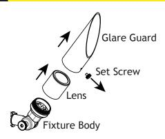
Loosen the set screw on the glare guard and remove it from the lens. Then twist and remove the lens from the fixture.
