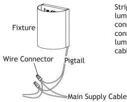
Strip both leads from the luminaire pigtail. Using two wire connectors (sold separately), connect the leads from the luminaire to the main supply cable leads.
