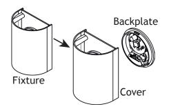
Rotate the cover clockwise until it is stops and then lift the cover straight off.
