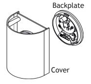
Push the shade hard onto the backplate aligning the gaps (air tighten moisture proof fixtures require some force to get the air out). Once the shade is flush with the backplate, rotate the shade until it stops and locks into place.
