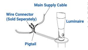
Strip both leads from luminaire pigtail. Using two UL listed wire connectors (sold separately), connect the leads from the luminaire to main supply cable leads.
