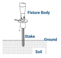
Insert the stake into the desired soil until flange of stake is flush to the ground.
