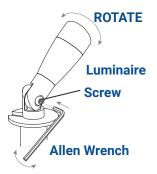
By using the Allen wrench, loosen the screw at the knuckle and adjust the luminaire to the desired direction. Once the desired direction is achieved, tighten the screw.
