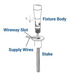
Pass the supply wires of the fixture body through the wireway slot on the stake. Thread the fixture body onto the stake.
