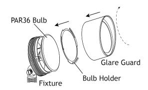
Tuck the excess wires inside of the fixture and place the PAR36 bulb inside. Place the bulb holder onto the top of the PAR36 bulb and thread the glare guard onto the fixture.
