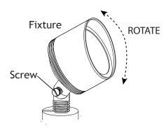
Loosen the knuckle and adjust the fixture to the desired orientation. Tighten the knuckle after you find the desired orientation.
