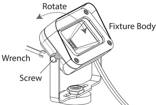
Adjust the fixture body to the desired orientation and tighten the screws with the wrench.
