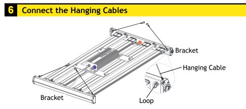
Attach the hook of the hanging cable to the loop on the bracket.
