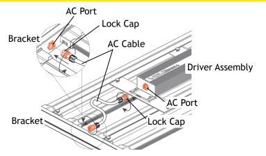
Connect one end of the AC power cable to the AC port on the bracket and connect the other end of the AC power cable to the AC port on the driver assembly. Tighten the lock caps on the connectors.
