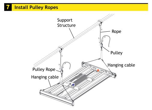
Hang the pulley ropes to the support structure by wrapping the pulley rope around the support structure and make a knot at the end of the rope. Attach the two hanging cables to the same hook on one pulley rope. Attach the rest of the hanging cables to the same hook on the other pulley rope. Adjust the ropes length on the pulley to level the LED fixture. The minimum hanging height of the LED fixture to the top of the target is the 6 inches.
