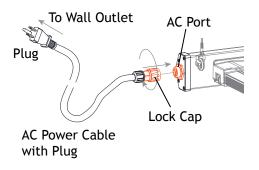
Connect the connector end of the AC power cable with plug to AC port on the bracket. Tighten the lock cap. Insert the plug on the other end of the AC power cord to the wall outlet.
