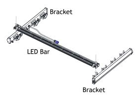
Place the two brackets on a flat working surface. Place the LED bar onto the brackets and press both ends down until they click. Repeat the process to assemble all LED bars onto the brackets.
