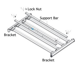
Flip the brackets over with the LED bars so that LED chips facing down. Attach the two support bars onto brackets and secure with the lock nuts. Hand tighten until snug.
