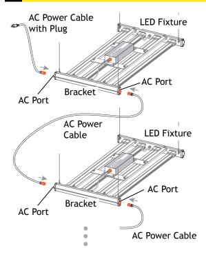
Connect the connector end of the AC power cable to the AC port on the bracket of the first LED fixture. Connect the second LED fixture to the first LED fixture by connecting the ends of the AC power cable to the AC ports. Repeat this process to connect more LED fixtures.
