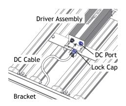
Connect the DC cable on the bracket to the DC port on the driver assembly. Tighten the lock cap on the connector.
