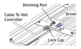
Connect the cable from Volt controller to dimming port on the driver. Tighten the lock cap.
