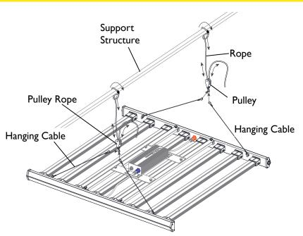
Hang the pulley ropes to the support structure by wrapping the pulley rope around the support structure and make a knot at the end of the rope. Attach the two hanging cables to the same hook on one pulley rope. Attach the rest of the hanging cables to the same hook on the other pulley rope. Adjust the ropes length on the pulley to level the LED fixture. The minimum hanging height of the LED fixture to the top of the target is the 12 inches.
