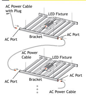
Connect the connector end of the AC power cable to the AC port on the bracket of the first LED fixture. Connect the second LED fixture to the first LED fixture by connecting the ends of the AC power cable to the AC ports. Repeat this process to connect more LED fixtures.
