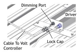
Connect the cable from Volt controller to dimming port on the driver. Tighten the lock cap.
