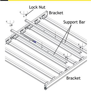
Flip the brackets over with the LED bars so that LED chips are facing down. Attach the two support bars onto brackets and secure with the lock nuts. Hand tighten until snug.
