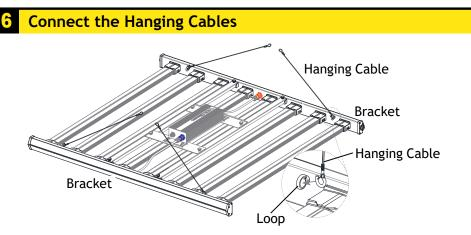
Attach the hook of the hanging cable to the loop on the bracket.
