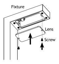
Place the lens back onto the fixture and secure with the previously removed screws. Tighten until snug.
