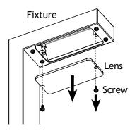
Remove the lens from the fixture by loosening the screws.
