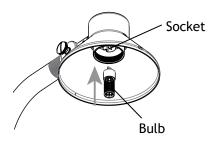
Insert the bulb with the correct wattage and type marked on the fixture label and push into place.
