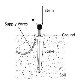
Pass the supply wires through the center hole of the stake and thread the stem onto the stake. Hand tighten until snug. Clear away an area in the ground and lay the supply wires into the wireway slot.
