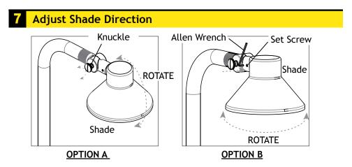
There are two methods to adjust the shade direction. NOTE: Do not rotate the shade a full 360°. This will damage the internal wiring.
