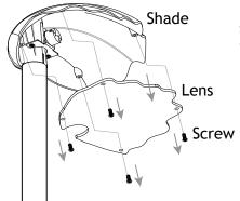
Using a screwdriver, loosen screws on the lens and remove the lens from the shade.
