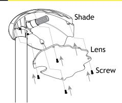
Place the lens back onto the shade and secure with previously removed screws. Tighten until snug with screwdriver.
