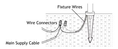
Strip two leads from fixture wires. Using two UL listed wire connectors (sold separately), connect leads from fixture wires to main supply cable leads.
