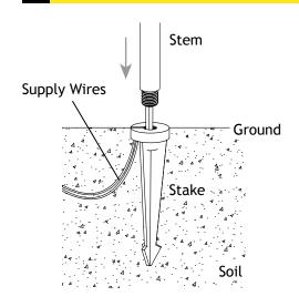
Pass supply wires through the center hole of the stake and thread the stem onto the stake. Hand tighten until snug. Clear away area in ground and lay supply wires into wireway slots.
