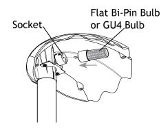
Insert bulb with correct wattage and type marked on fixture label and push into place.
