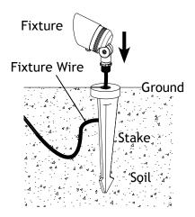
Pass the fixture wire through the center opening of the stake. Thread the fixture onto the stake. Hand tighten until snug.
