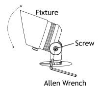
Using the Allen wrench, loosen the screw on the knuckle and adjust the fixture to your desired direction. Once your direction is achieved, tighten the screw until snug.
