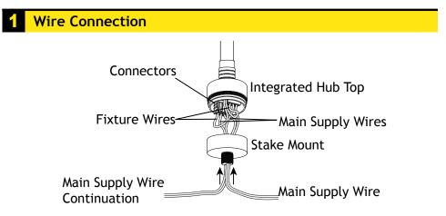
Insert the main supply wire continuation (if needed) and the main supply wire up through the bottom of the stake mount and strip the ends of both sets of supply wires.
