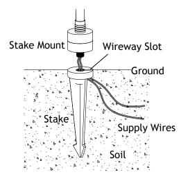
Clear away an area in the ground at the wireway slot on top of the stake. Lay the supply wires into the wireway slot and screw the stake mount on to the stake. Tighten until snug. INSTALLATION INSTRUCTIONS
