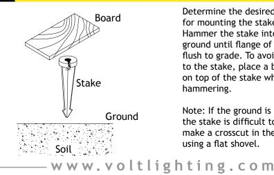
Determine the desired location for mounting the stake mount. Hammer the stake into the ground until flange of stake is flush to grade. To avoid damage to the stake, place a board on top of the stake while hammering.
