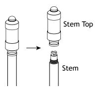
Twist the stem top counterclockwise and remove it from the stem.
