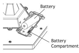
Insert the battery into the battery compartment.
