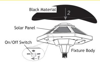
Slide the ON/OFF switch of the fixture to the "ON" position. Cover solar panels completely by using black materials. The fixture will light up when the solar panel is covered and turn back off when it is uncovered.
