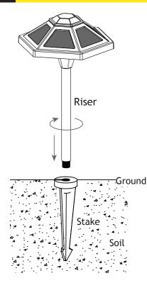
Thread the riser on to the stake and hand tighten until snug.
