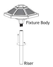
Thread the riser onto the fixture and hand tighten until snug.
