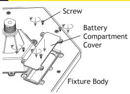
Place the battery compartment cover back onto the fixture body and secure with the previously removed screws.
