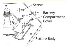
Using a screwdriver, remove the battery compartment cover from the fixture body.
