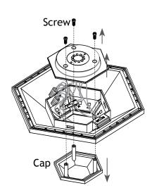
Using a screwdriver, remove the 3 screws. Then take the light source out of the hat.
