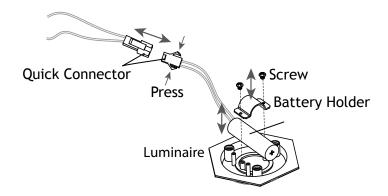
Disconnect the quick connector by pressing the tabs on the side. Remove the old battery by removing the two screws. Replace the battery and secure it with the previously removed screws. Then connect the tabs of the quick connector back together.
