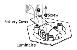
Remove the battery cover from the luminaire by using a screwdriver and removing the screws.
