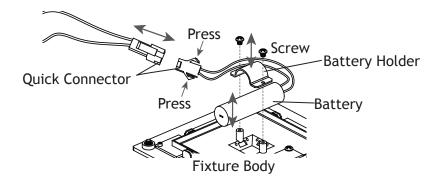
Disconnect the quick connector by pressing the tabs on the side. Remove the old battery by removing the two screws. Replace the battery and secure it with the previously removed screws. Then connect the tabs of the quick connector back together.
