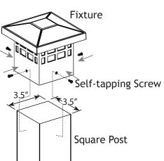
Attach the fixture onto a 4"x 4" square wood post and secure with self-tapping screws.
