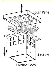
Using a screw driver, remove the screws from the corners to remove the solar panel from the fixture body.
