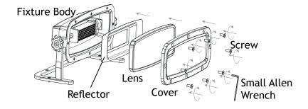
Place the reflector, the lens and the cover back onto the fixture body and secure with previously removed screws. Hand tighten until snug with Small Allen Wrench.
