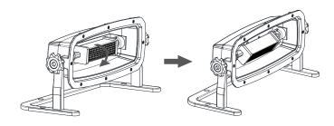
If you would like to decrease the output, rotate the R7S bulb towards the back of the fixture.
