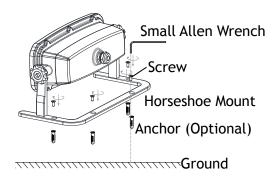
Attach the horseshoe mount to the desired location and mark (4) points for anchors from the holes on the horseshoe mount. Drill proper holes on the location and insert the anchors into the drilled holes. Attach the horseshoe mount onto the anchors. Thread the mounting screws into the anchors to secure the horseshoe mount. Hand tighten until snug with Small Allen Wrench.
