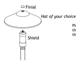
Place the hat of your choice onto the stem top and secure it with the finial. Hand tighten until snug.
