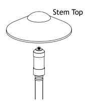
**Note:** For Cast Brass hats you will not need a finial to install the hat. You will screw the hat directly to the top of the stem.
