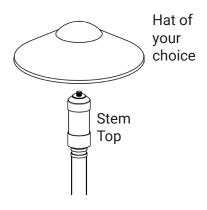
Thread the hat of your choice onto the stem top. Hand tighten until snug.
