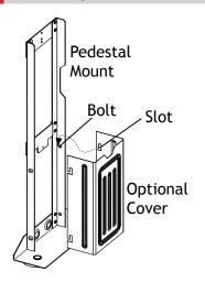
Fit all the slots on the optional cover to the bolts on the pedestal mount.
