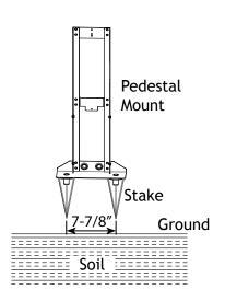
Determine the desired location for mounting the pedestal. Push the stakes of the pedestal mount into the ground until flange of stake is flush to grade. The easiest way to do this is with your foot directly over the bracket the stake is attached to.
