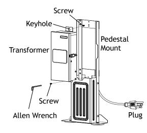
Start by removing the upper screw from the pedestal mount. Next, loosen the lower screw on the pedestal mount enough to allow the transformer tab to sit on it. This should hold the transformer in place. Carefully hold the transformer steady and reinstall the upper screw to secure the transformer into place. Finally, tighten both set screws until snug.
