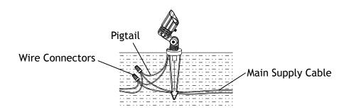
Strip both leads from the luminaire pigtail. Using two wire connectors (sold separately), connect the leads from the luminaire to the main supply cable leads.
