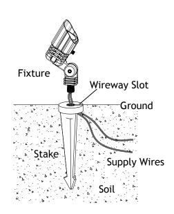
Clear away an area in the ground at the wireway slot on top of the stake. Lay the fixture pigtail into the wireway slot and attach the fixture onto the stake. Tighten until snug.
