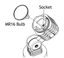
Insert MR16 bulb with the correct wattage and type marked on the fixture label.
