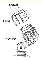
Place the lens back onto the fixture and rotate it until it is secured properly.
