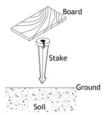
Determine the desired location for mounting the stake mount. Hammer the stake into the ground until flange of stake is flush to grade. To avoid damage to the stake, place a board on top of the stake while harmmering.
