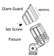
Loosen the set screw and remove the glare guard from the fixture.
