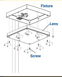
Remove the lens from the fixture.
