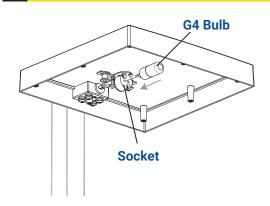
Insert G4 bulb with correct wattage and type marked on fixture label.
