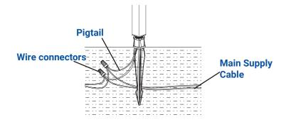
Strip both the leads from the luminaire pigtail. Using two UL listed wire connectors (sold separately), connect the leads from the luminaire to the main supply cable leads.
