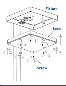
Place the lens back onto the fixture and secure with previously removed screws.
