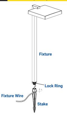
Pass the fixture wire through the stake and thread the stake onto the fixture. Thread the lock ring against the stake and hand tighten until snug.
