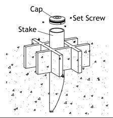
Remove the cap from the stake by loosening the set screws.
