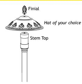
Place the hat of your choice onto the stem top and secure it with the finial, or thread the hat of your choice onto the stem top directly. Hand tighten until snug.
