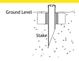
Dig a hole in the ground for the stake. Slide the stabilizer grid onto the stake and secure with the screws. Place the stake and backfill against the mounting stake.
