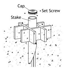
Remove the cap from the stake by loosening the set screws.
