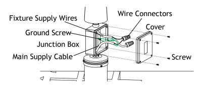
Strip the leads from the fixture supply wire and main supply cable. Using wire connectors (sold separately), connect the leads from the fixture supply wire to the main supply cable leads. Then, connect the ground wires to the ground screw in the junction box.
