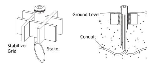
Dig a hole in the ground for the conduit runs and the stake. Install the conduit. Slide the stabilizer grid onto the stake and secure with the screws. Place the stake over the conduit runs then backfill against the mounting stake.
