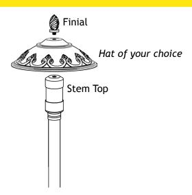
Place the hat onto the stem top and secure it with the finial, or thread the hat onto the stem top directly. Hand tighten until snug.
