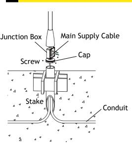
Pass the main supply cable into the junction box. Place the cap back onto the stake and secure with the previously removed screws. Tighten until snug with a screwdriver.
