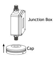
Thread the cap onto the Junction Box.
