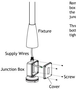
Remove the cover from the junction box by loosening the screws. Place the fixture supply wires into the junction box.
