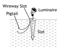
Clear away an area in the ground at the wireway slot on top of the stake. Lay the luminaire pigtail into the wireway slot and attach the luminaire onto the stake. Tighten until snug.
