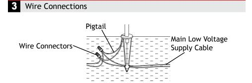
Strip both leads from the luminaire pigtail. Using two wire connectors (sold separately), connect the leads from the luminaire to the main supply cable leads.
