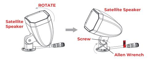
Adjust the satellite speaker to the desired direction. Using the Allen wrench, tighten the screw at the joint to secure the satellite speaker angle.
