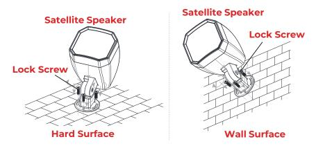
Place the satellite speaker on a hard surface or wall surface. Drill the screws through mounting holes to secure the satellite speaker.
