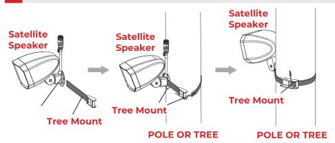
**NOTE:** The maximum width of the tree mount is 30mm (1.18"). Pass the tree mount (not included) through the gap on the base. Wrap the tree mount around the desired pole or tree and fasten to secure the satellite speaker.
