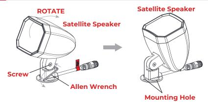
Use the Allen wrench, loosen the screw at the joint of the satellite speaker. Do NOT remove the screw. Rotate the satellite speaker to expose the mounting holes on the base.
