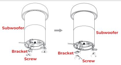
Loosen the screws to remove the brackets from the bottom of the subwoofer. Reverse the brackets and install them back to the bottom of the subwoofer. Secure with previously removed screws.
