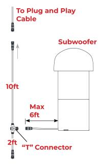
The DVC subwoofer comes prewired with a 6ft of cable. The distance from the subwoofer to the "T" connector on the plug and play cable is maximum 6ft.
