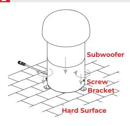
Place the subwoofer on a hard surface. Pass the screws through holes on the bracket and drill them into the hard surface to secure the subwoofer.
