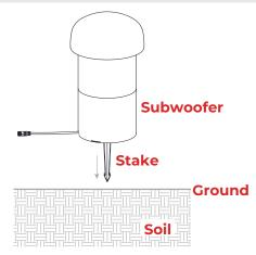
Insert the stake into the ground until the bottom of the subwoofer flush to the ground.
