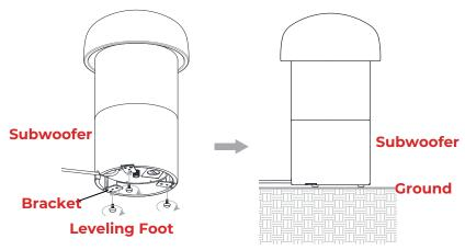
Thread the leveling feet onto the bottom bracket of the subwoofer.
