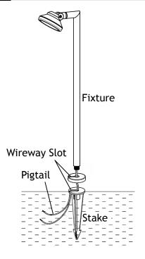
Clear away an area on the ground at the wireway slot on top of the stake. Lay the luminaire pigtail into the wireway slot and thread the fixture onto the stake. Tighten until snug using the lock nut to secure it to the base.
