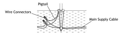
Strip both leads from the luminaire pigtail. Using two wire connectors (sold seperately), connect the leads from the luminaire to the main supply cable leads.
