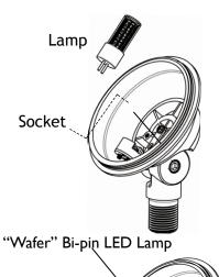
Insert the lamp with the correct wattage and type marked on the fixture label.
