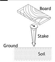
Determine the desired location for mounting the fixture. Hammer the stake into the ground until the flange of the stake is flush to grade. To avoid damage to the stake, place a board on top of the stake while hammering.
