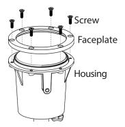
Loosen the screws and remove the faceplate from the housing.
