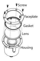
Place the lens, gasket, and faceplate back onto the housing. Secure them with the screws previously removed. Hand tighten until snug, then use a srewdriver to secure them in a star pattern.
