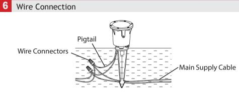
Strip both leads from the luminaire pigtail. Using two wire connectors (sold seperately), connect the leads from the luminaire to the main supply cable.
