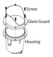
Attach the glare guard onto the housing and secure with the screws previously removed.
