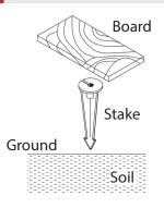
Determine the desired location for mounting the fixture. Hammer the stake into the ground until flange of stake is flush to grade. To avoid damage to the stake, place a board on top of the stake while hammering.
