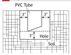
Dig a hole in the ground making sure there is approximately 3 inches of room on all sides surrounding the PVC tube for pea gravel or sand.
