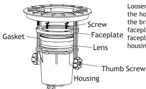
Loosen the thumb screws and slide the housing down to the end of the brackets. Then untighten the faceplate screws and remove the faceplate, gasket, and lens from the housing.
