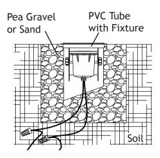
Install the PVC tube with the fixture in the hole and fill the extra space with pea gravel or sand for proper water drainage.
