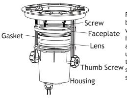
Place the lens, gasket, and faceplate back onto the housing. Secure them with the screws previously removed. Hand tighten until snug, then use a screwdriver to secure the screws using a star pattern. Adjust housing to your desired height and angle, then secure it in place with the thumb screws.
