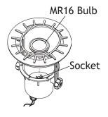
Insert the bulb with the correct wattage and type marked on the fixture label.
