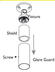
Use a screwdriver to unlock the screw. Then, remove the glare guard from the shield. Next, remove shield from the fixture.
