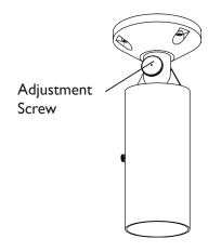
Loose adjustment screw and adjust lamp to your desired angle and then tighten adjustment screw.
