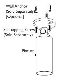
Determine your desired location for the fixture. Pass self-tapping screws through the holes on the surface mount. Thread self-tapping screws into wall surface to secure the fixture.
