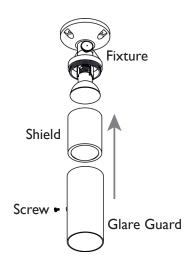
Replace the shield over the lamp and thread onto the fixture. Tighten until snug. Attach the glare guard back onto the shield and secure with the screw. Tighten until snug with a screwdriver.
