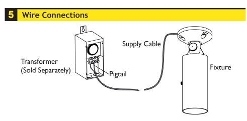
Lay out the supply cable to the transformer. Strip two leads from luminaire pigtail. Connect leads from luminaire supply cable to transformer (sold separately).
