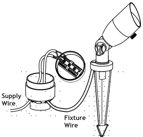
C. Run the fixture wire to the hub and insert the wire through the rubber grommets on the bottom of the hub. Then, flip one of the terminal levers open, insert one end of the stripped fixture wire, and flip the lever closed to make your connection. Last, flip the lever open that is directly opposite from the first fixture wire connection, on the other side of the terminal block, and insert the other end of the fixture wire and flip the lever closed to make the connection.
