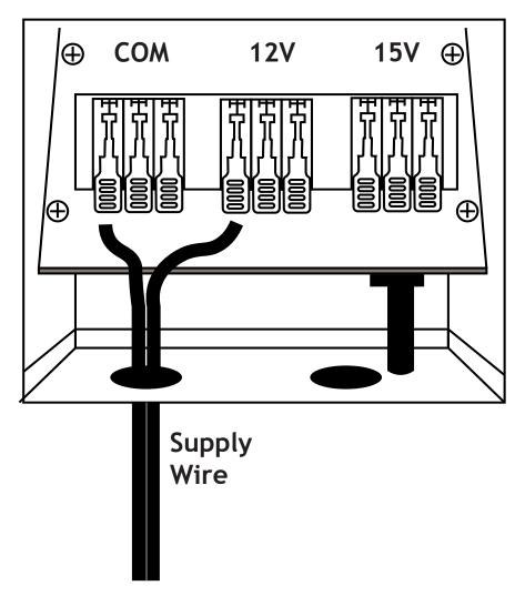
B. Run the supply wire to the centrally located hubs and insert the wire through the rubber grommets on the bottom of the hub. Then, flip one of the terminal levers open, insert one end of the stripped supply wire, and flip the lever closed to make your connection. Last, flip the lever open that is directly opposite from the first connection, on the other side of the terminal block, and insert the other end of the supply wire and flip the lever closed to make the connection.
