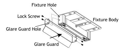
Attach the glare guard onto the fixture body by aligning the holes of the glare guard to the holes on the side of the fixture body and secure them with the lock screws. Tighten with a screw driver.
