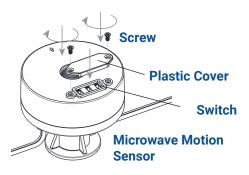
Place the plastic cover back on top of the switches and secure with the previously removed screws.
