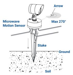
Aim the arrow on the microwave motion sensor to the desired detective area. The maximum detective range is 270°.
