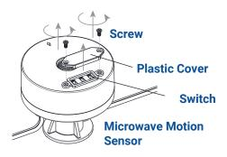
Using a screwdriver, remove the plastic cover from the switch on top of the sensor.
