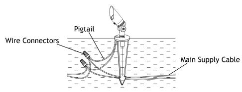
Strip both leads from the luminaire pigtail. Using two wire connectors (sold separately), connect the leads from the luminaire to the main supply cable leads.
