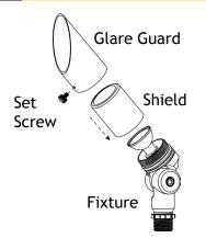
Unlock the set screw and remove the glare guard from the shield. Loosen the shield and remove it from the fixture.
