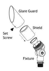
Attach the shield back onto the fixture. Place the glare guard over the shield and secure with the set screw. Tighten until snug.
