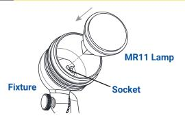
Insert the MR11 lamp with correct wattage and type marked on fixture label.
