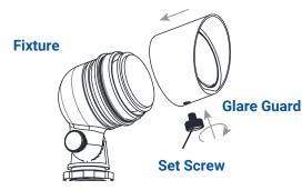
Place the glare guard back onto the fixture and secure with previously removed set screw.
