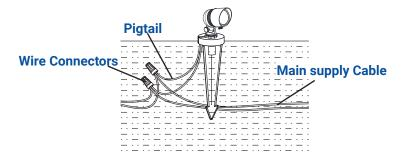
Strip both the leads from the luminaire pigtail. Using two UL listed wire connectors (sold separately), connect the leads from the luminaire to the main supply cable leads.
