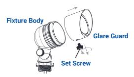
Loosen the set screw and remove the glare guard from the fixture.
