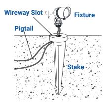
Clear away an area in the ground at the wireway slot on top of the stake. Lay the luminaire pigtail into the wireway slot and screw the fixture on to the stake. Tighten until snug.
