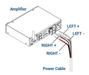
Plug in the male color coded cable end to the female of the same color on the amplifier.
