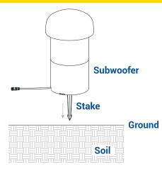
Insert the stake into the ground until the bottom of the subwoofer flush to the ground.
