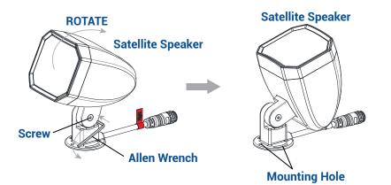
Use the Allen wrench, loosen the screw at the joint of the satellite speaker. Do NOT remove the screw. Rotate the satellite speaker to expose the mounting holes on the base.
