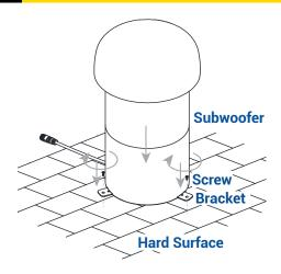
Place the subwoofer on a hard surface. Pass the screws through holes on the bracket and drill them into the hard surface to secure the subwoofer.
