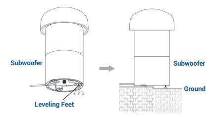
Adjust the feet as needed to ensure the subwoofer is level. For the best stability, place the subwoofer on a flat surface.
