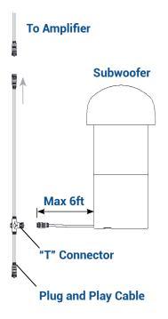
The DVC subwoofer comes prewired with a 6ft of cable. The distance from the subwoofer to the "T" connector on the plug and play cable is maximum 6ft.
