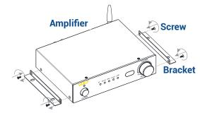
Attach the brackets to the sides of the amplifier and secure with previously removed screws.
