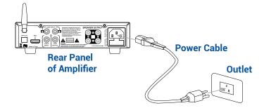
Connect the amplifier to the outlet by using the provided power cable. Once powered up, the blue Bluetooth light will start blinking. Access the Bluetooth icon on your Smartphone. Select "AU-AMP" from the selective choices. Once the blue light stops blinking and turns to a solid blue, your smartphone & amplifier are paired together.
