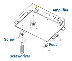
Using a screwdriver remove the feet from the amplifier.
