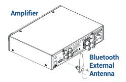
Unbox the amplifier. Thread the bluetooth external antenna to the back of the amplifier. The amplifier can be placed directly onto a flat surface or fix mounted. Refer to steps 2 through 5 for installation instructions if you want to use the fixed mount.
