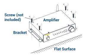
Place the amplifier onto a flat surface. Secure by drilling the screws into both sides of the brackets..
