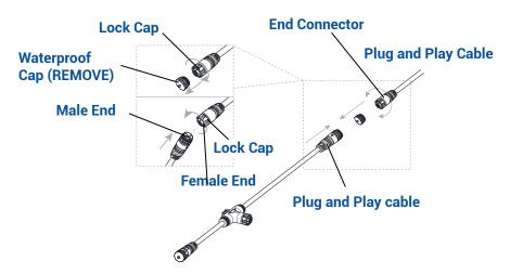
Connect the subwoofer and the desired plug and play cable together.
