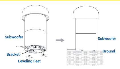
Thread the leveling feet onto the bottom bracket of the subwoofer.
