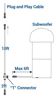
The DVC subwoofer comes prewired with a 6ft of cable. The distance from the subwoofer to the "T" connector on the plug and play cable is maximum 6ft.
