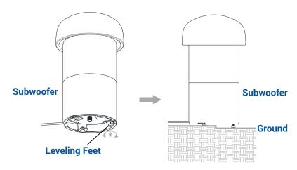
Adjust the feet as needed to ensure the subwoofer is level. For the best stability, place the subwoofer on a flat surface.
