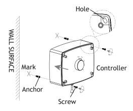
Place the controller on to the wall surface and mark two points on the wall using the two corner holes. Remove the controller and drill holes for the anchors using the marks as a guide. Insert the anchors into the drilled holes.
