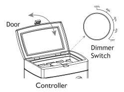
Open the door of the cover. Rotate the dimmer switch to adjust the LED lumens (PPF).
