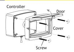
Attach the cover back onto the controller properly. Open the door of the cover and install four screws into the holes at the corners. Tighten the four screws with a screwdriver to secure the cover to the controller. Close the door after installation.
