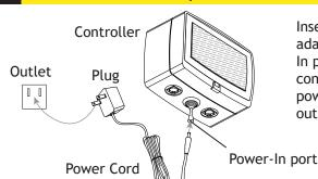
Insert the end of the power adaptor cord into the Power-In port on the controller and connect the plug end of the power adaptor to the wall outlet.
