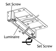
Using an Allen Key, loosen the set screws on the side of the fixture to rotate the luminaire to your desired direction by hand. Once you have the desired angle, tighten down the set screws with the Allen Key.
