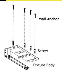
Place the fixture body onto the desired location. Mark four points on the mounting surface using the holes of the mount as a guide. Set the fixture aside and drill the proper holes where you placed the marks then insert the wall anchors into the drilled holes. Place the fixture onto the surface and secure with screws using a screwdriver.
