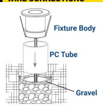
Place the PC tube into the hole and fill gravel around the PC tube properly.
