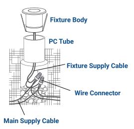
Pass the fixture supply cable from the fixture body through the PC tube. Strip both leads from fixture supply cable. Using two UL listed wire connectors (sold separately), connect leads from fixture supply cable to main supply cable leads.
