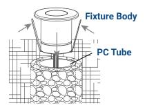
Push the fixture body into the PC tube until the flange of fixture body is flush to the top of the PC tube.
