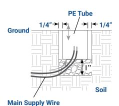
Dig a 1.76" diameter, 2.38" deep hole in the ground. Run supply wires up through the bottom of the PC tube. Place 1" of gravel in the bottom of hole for proper drainage.
