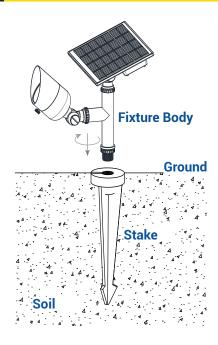
Insert the fixture onto the stake.
