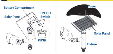
Turn the ON-OFF switch to ON. Cover the panel. The fixture will light up when the solar panel is covered and turn back off when it is uncovered.
