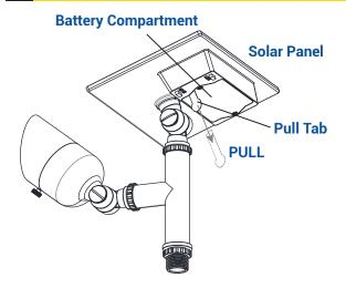
Remove the pull tab out of the battery compartment on the bottom of the fixture.
