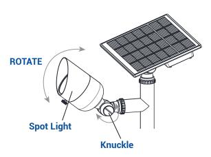
Loosen the knuckle of the spot light. Adjust the spot light to the desired direction. Tighten the knuckle to hold the spotlight in place.
