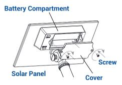
Place the cover back onto the battery compartment and secure with previously removed screws. Tighten with a screwdriver.
