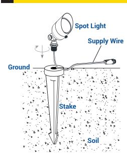
Clear away an area in the ground at the wireway slot on top of the stake. Lay the spot light supply wire into the wireway slot and screw the solar panel on to the stake.
