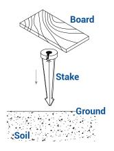
Determine the desired location for mounting the solar panel. Hammer the stake into the ground until flange of stake is flush to grade. To avoid damage to the stake, place a board on top of the stake while hammering.
