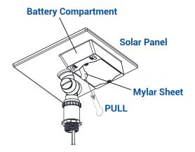
Remove the pull tab out of the battery compartment on the bottom of the fixture.
