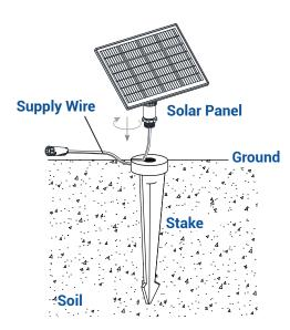
Clear away an area in the ground at the wireway slot on top of the stake. Lay the solar panel supply wire into the wireway slot and screw the solar panel on to the stake.
