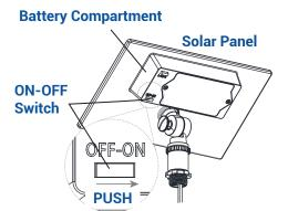
Turn the ON-OFF switch to ON.
