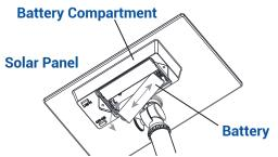
Replace the battery with correct specifications as below:
