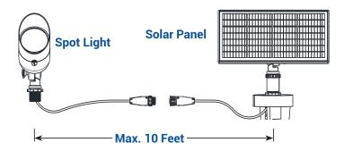
Decide the installation position of the spot light. The distance between the spot light to the solar panel should be less than 10 feet.
