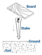
Determine the desired location for mounting the spot light. Hammer the stake into the ground until flange of stake is flush to grade. To avoid damage to the stake, place a board on top of the stake while hammering.
