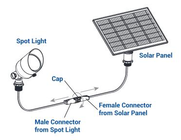
Loosen the cap on the female connector to disconnect the male connector from the spot light to the female connector from solar panel.
