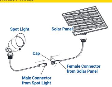
Connect the male connector from the sport light to the female connector from solar panel. Screw the cap on the female connector.
