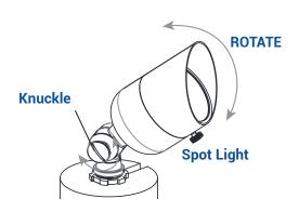
Loosen the knuckle of the spot light. Adjust the spot light to the desired direction. Always tighten the knuckle after your desired direction is achieved.
