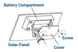
Loosen the screws on the back of the solar panel to remove the cover from the battery compartment.
