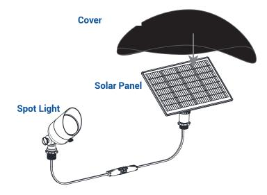
Cover the panel. The fixture will light up when the solar panel is covered and turn back off when it is uncovered.
