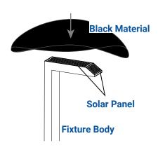
Cover solar panels completely by using black materials. The fixture will light up when the solar panel is covered and turn back off when it is uncovered.
