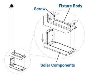
Remove the screws to separate the solar components from the fixture body.
