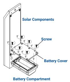
Place the battery cover back onto the battery compartment and secure with previously removed screws.
