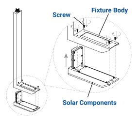
Place the solar components back into the fixture body and secure with previously removed screws.
