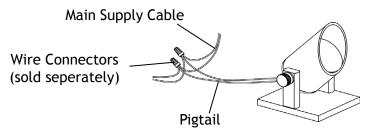
Place fixture body on your desired location. Strip both leads from luminaire pigtail. Using two wire connectors (sold seperately), connect the leads from the luminaire to the main supply cable leads. Make this connection at least 10' outside of the water.
