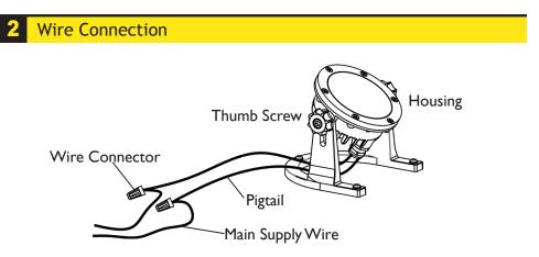
Strip both leads from the luminaire pigtail. Using wire connectors (sold seperately), connect the leads from the luminaire to the main supply cable leads.
