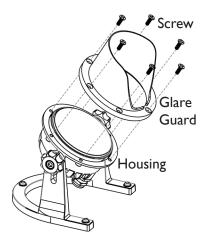
Install the glare guard onto the housing and secure it with the screws previously removed, tightening them in a star pattern.
