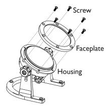
Loosen the screws on the faceplate and remove the faceplate from the housing.
