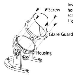
Install the glare guard onto the housing and secure it with the screws previously removed, tightening them in a star pattern.
