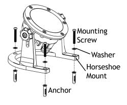
Place the horseshoe mount on the desired location and mark (3) points for the anchors from the holes on the horseshoe mount.
