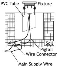
Place the fixture onto the PVC Tube. Pass the luminaire pigtail through the PVC tube.
