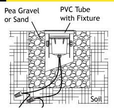
Install the PVC tube with fixture in the hole and fill the extra space with pea gravel or sand for proper water drainage.
