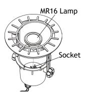
Insert the lamp with the correct wattage and type marked on the fixture label.
