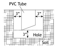
Dig a hole in the ground making sure there is approximately 3 inches of room on all sides surrounding the PVC tube for pea gravel or sand.
