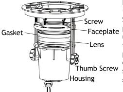
Place the lens, gasket and faceplate back onto the housing. Secure them with the screws previously removed. Hand tighten until snug, then use a screwdriver to secure the screws using a star pattern. Adjust housing to your desired height and angle, then secure it in place with the thumb screws.
