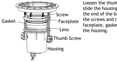
Loosen the thumb screws and slide the housing down to the end of the bars. Unscrew the screws and remove the faceplate, gasket, and lens from
