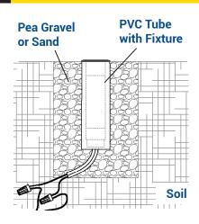
Install the PVC tube with fixture in the hole and fill hole with pea gravel or sand.
