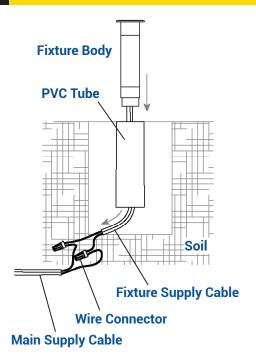
Pass the fixture wire through the PVC tube. Place the fixture body into the PVC tube.
